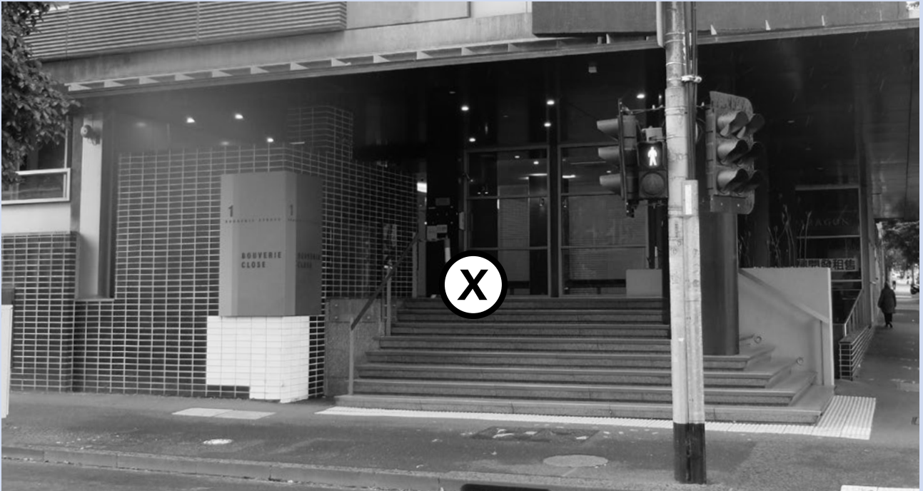
Figure 44: A tall staircase creates a psychological barrier and a blank wall does not relate positively to the street.
