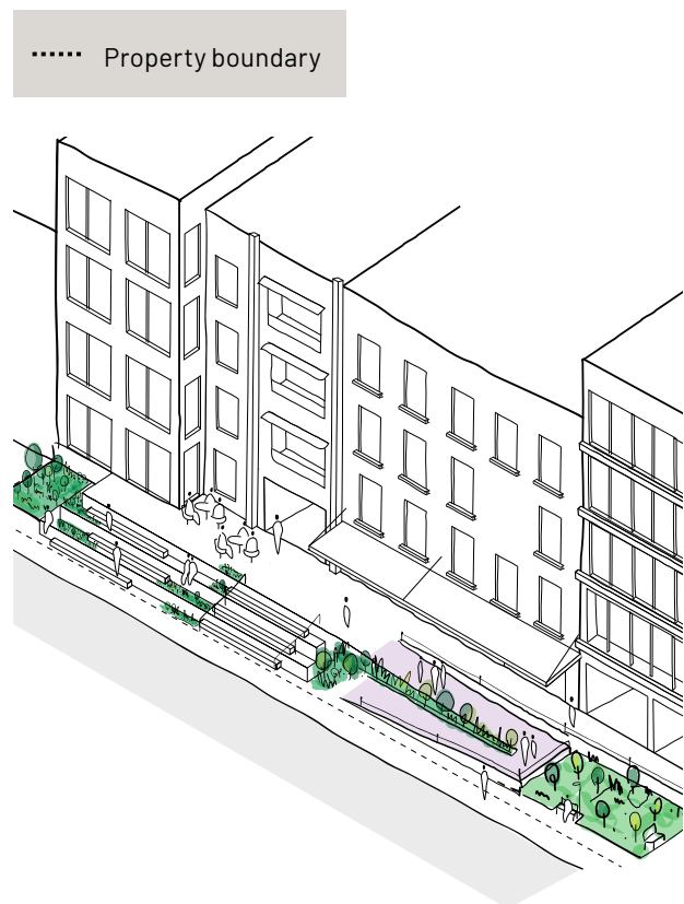
Figure 38: Elements such as terracing, seating, landscape bridge the visual gap between the elevated ground and street level and contribute to the activity and attractiveness of the streetscape.
