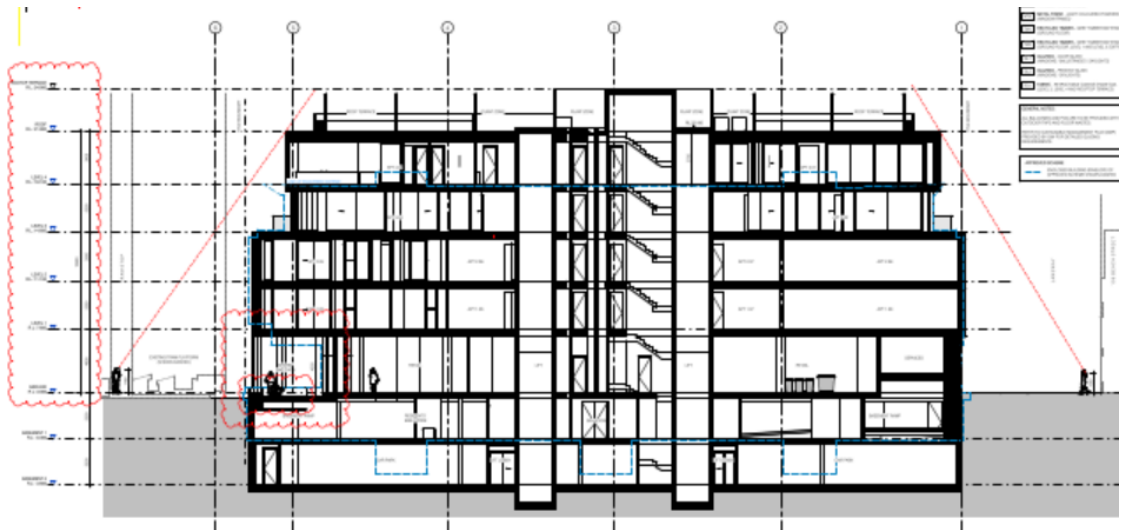
Fig 5: Section plan from the submitted architectural plans showing the setbacks from the side boundaries
