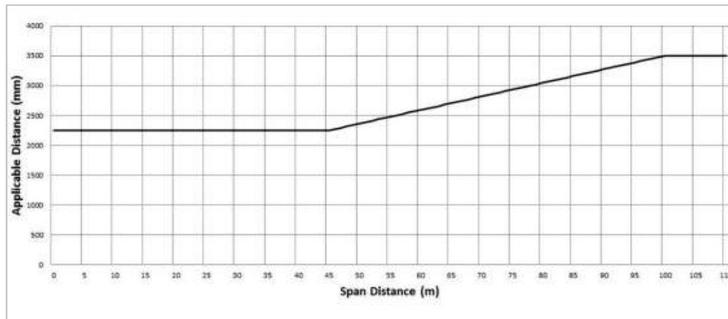
Graph 4: Uninsulated 66,000 Volt Electric Line in Low Bushfire Risk Area
