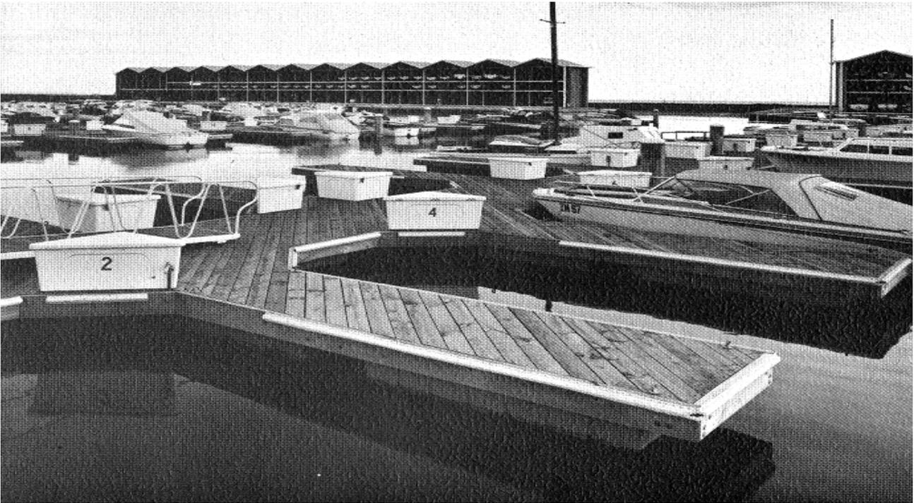
Figure 6: View of newly-completed marina, showing south dry boat storage building in background. Note floating berths, with diagonal timber decking, canted corners and triangular dock-boxes
