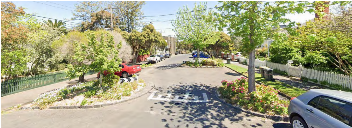
Grosvenor Street demonstrates another option for configuration of chicanes that requires vehicles to slow and let oncoming traffic pass (Image Credit Google Street View).
