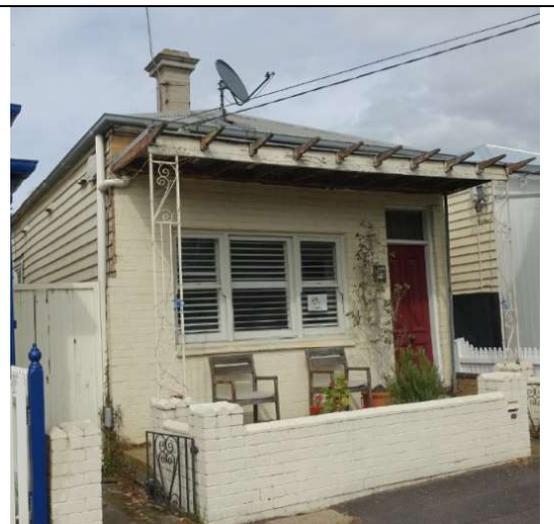
*Figure 48. 133 Farrell Street. Alterations: removal of eaves brackets, verandah, reformatting front window, and recladding front façade with cream brick.*
