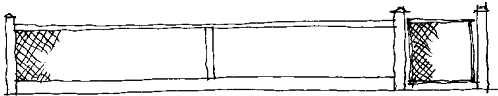
Chain wire mesh fixed to a wooden frame. From 800mm to 1000mm high.
