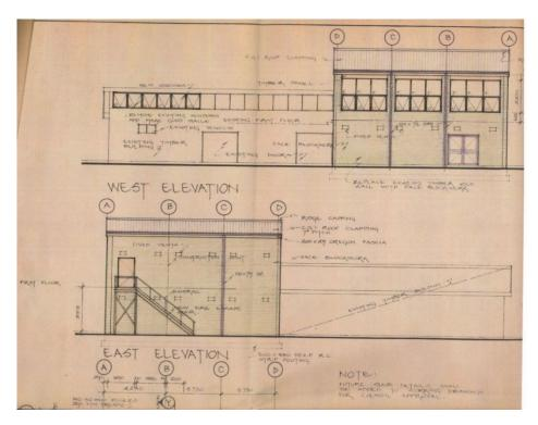
Figure 13. Detail of east and south elevations (note that south elevation is labelled west in these drawings), dated 1975, showing proposed face blockwork (Source: City of St Kilda)
