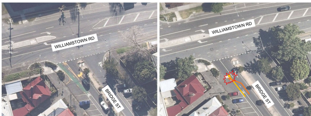
Image 1 Intersection of Bridge Street and Williamstown Road, Port Melbourne. Pop up bike lane (left image) and pre-existing conditions (right image) highlighting risk reintroduction.
