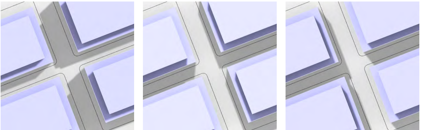
Overshadowing of a 20 m wide north-south street at 10.00 am, 12.00 pm and 2.00 pm based on a 4 storey street wall, 5 m upper level setback and 6 storey building height for non-residential development.
