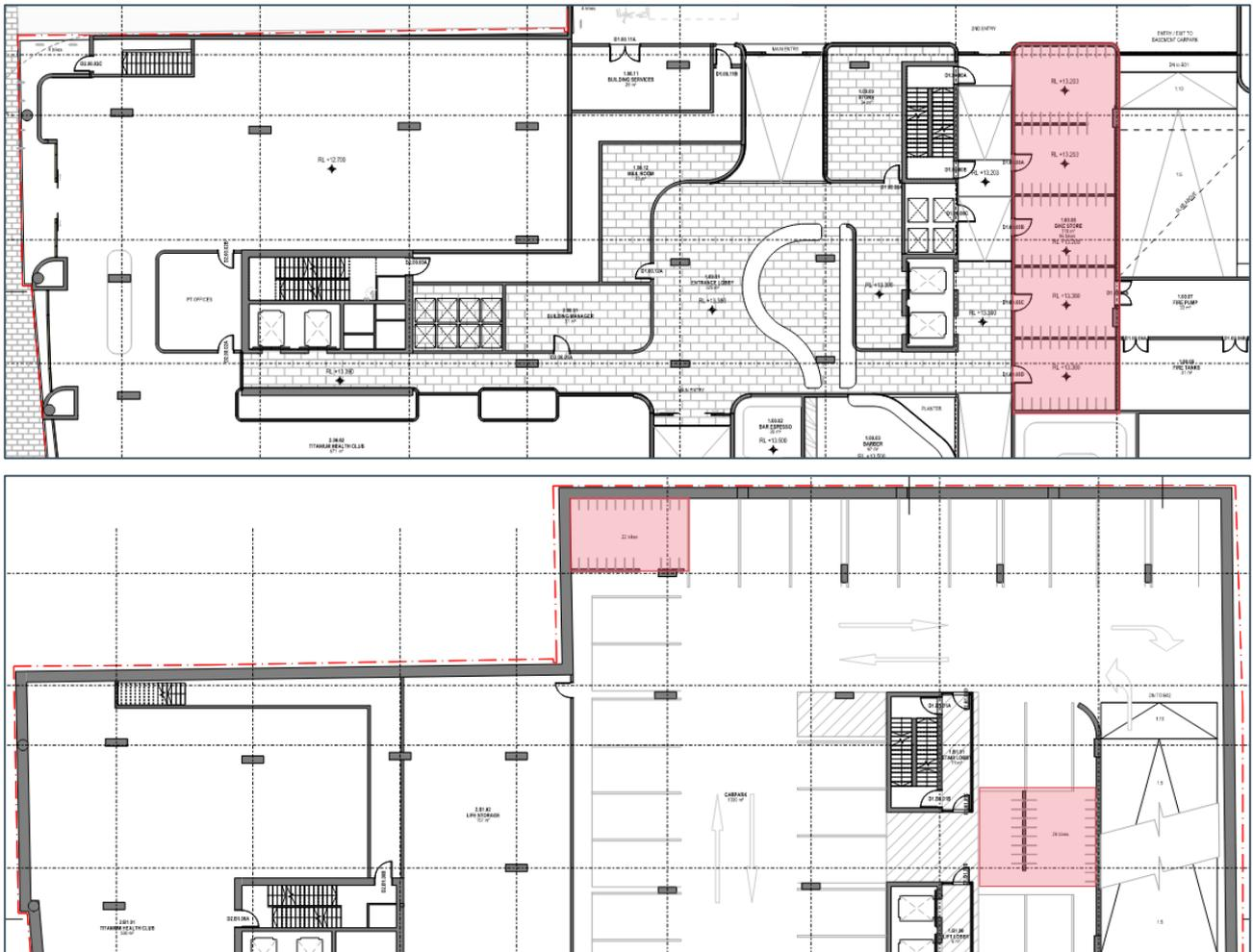
Figure 5 Bike parking facilities; ground floor (top), basement levels (bottom)
