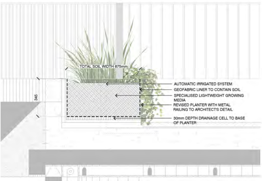
02. TOWER PLANTER - TYPICAL DETAIL - 1:20
