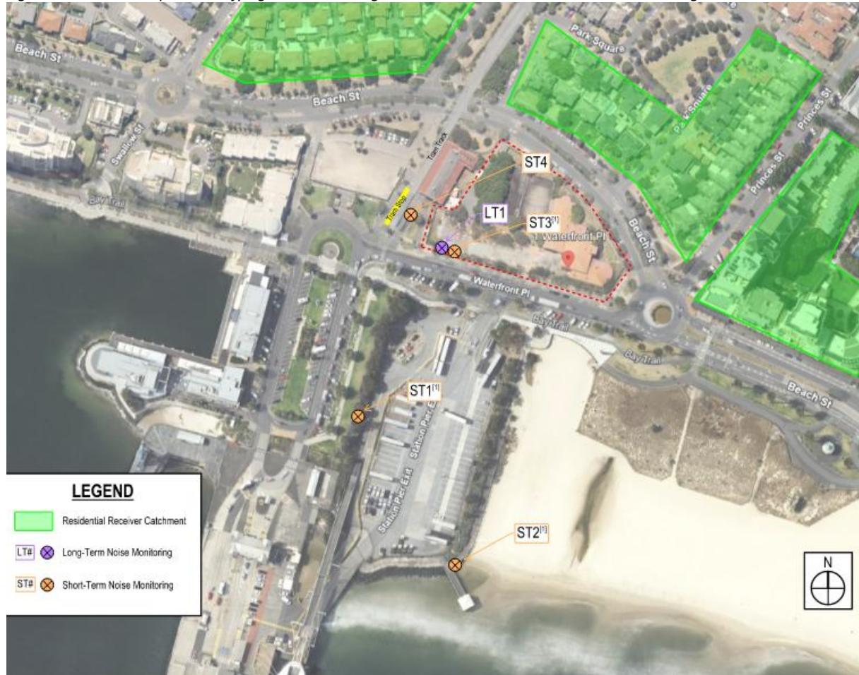
Figure 1: Acoustic site plan identifying the surrounding noise-sensitive receivers and noise monitoring locations
