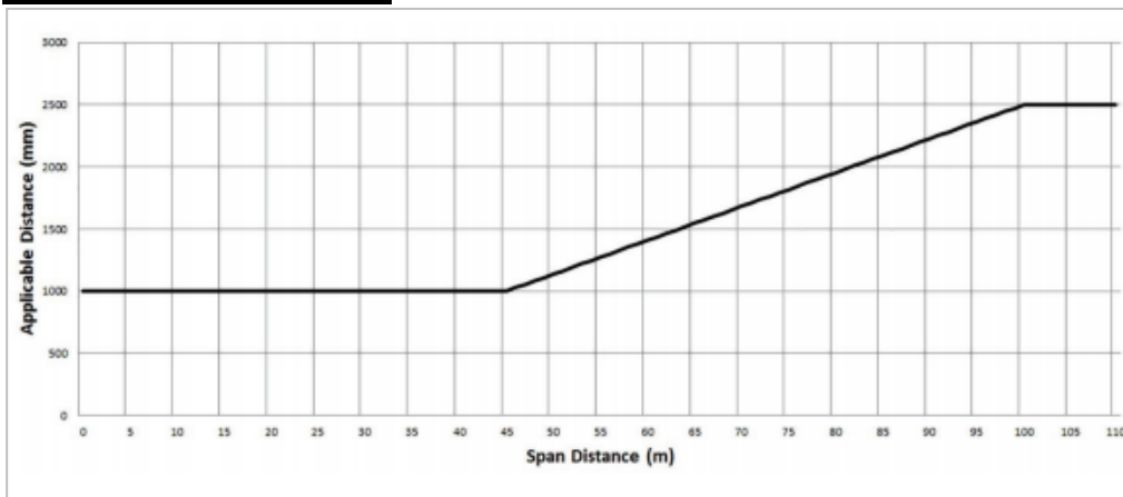
Graph 2: Uninsulated Low Voltage Electric Line in Low Bushfire Risk Area
