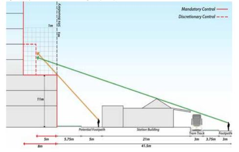
Figure 18 | The Railway Station interface setback diagram (above).
