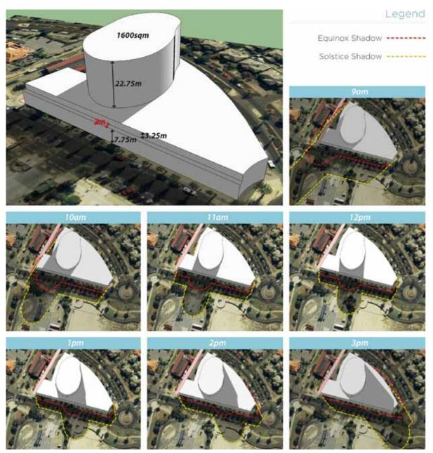
Figure 20 | Shadow diagram showing a possible development scenario on 22nd June (winter solstice shadow shown as yellow hatched line).
