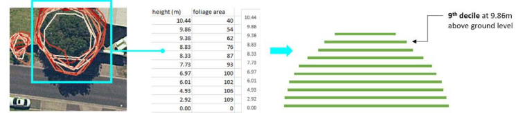
3 Canopy profile derived from LiDAR. Vertical extent of the canopy is divided into 10 sections (deciles) and is attributed with its corresponding area (sqm). The height of the 9 th decile is used to attribute tree height.
