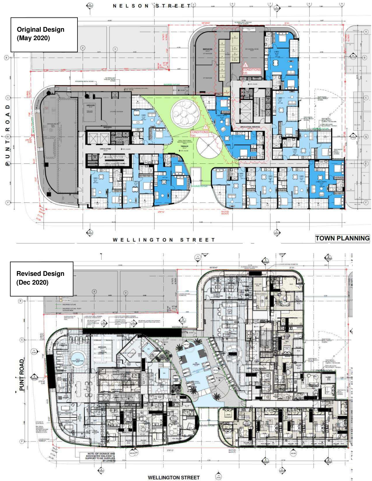
Figure 3: Podium rooftop (Level 03) plans for the development at One Wellington, St Kilda – comparison between revised design and original design tested in the wind tunnel
