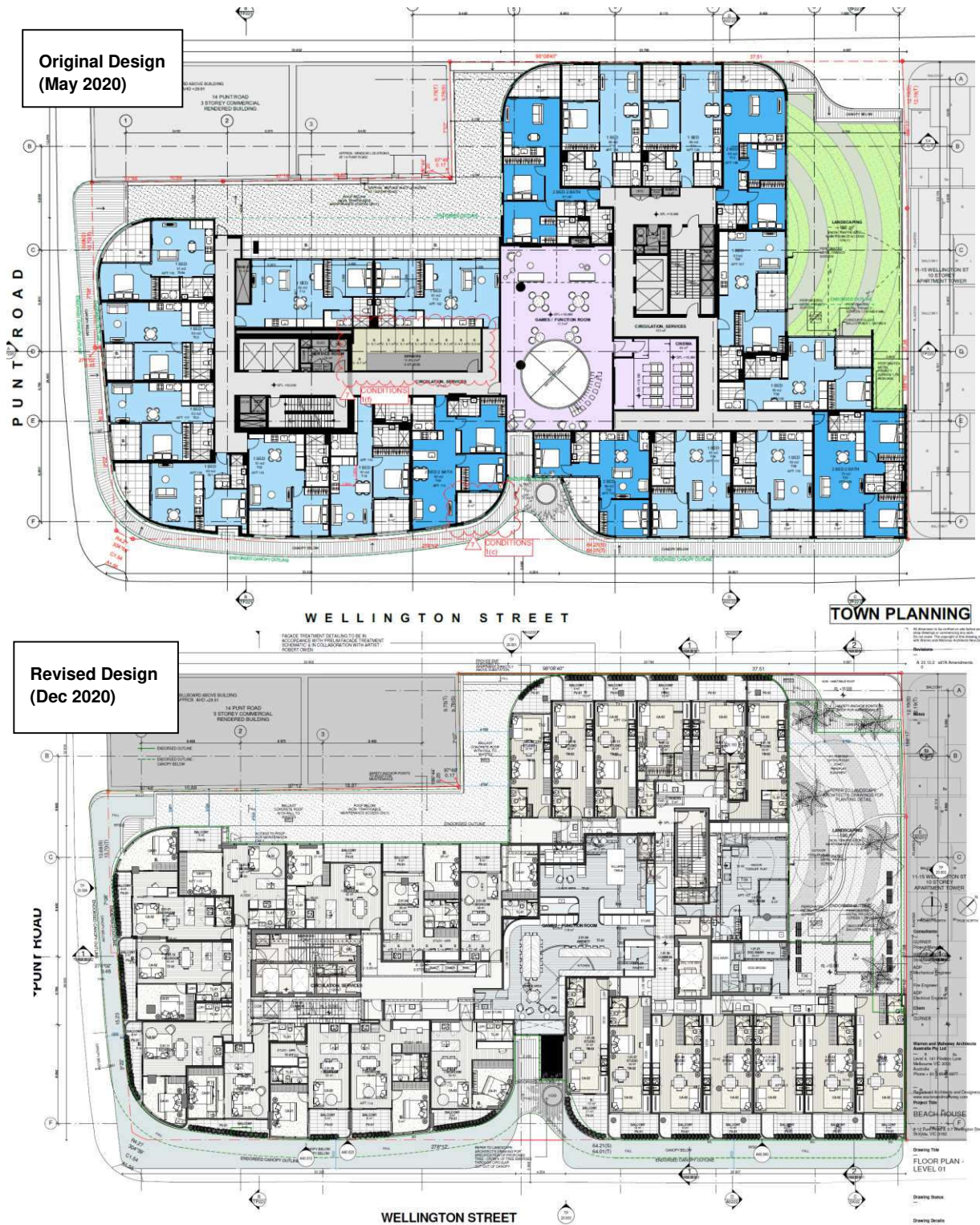
Figure 2: Level 01 floor plans for the development at One Wellington, St Kilda – comparison between revised design and design tested in the wind tunnel
