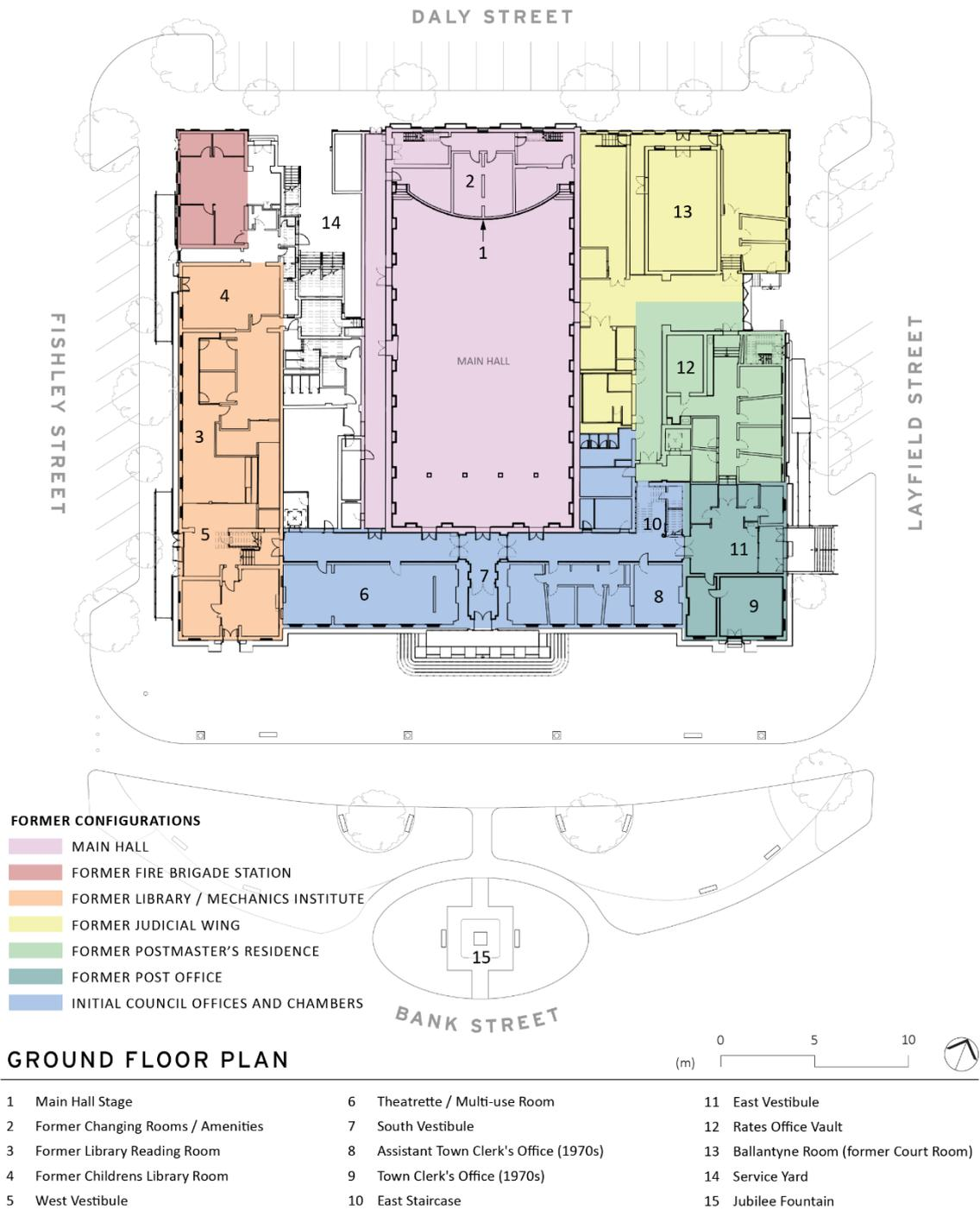
Figure 15 Existing conditions ground floor plan overlaid with locations (approximate) of original functions
