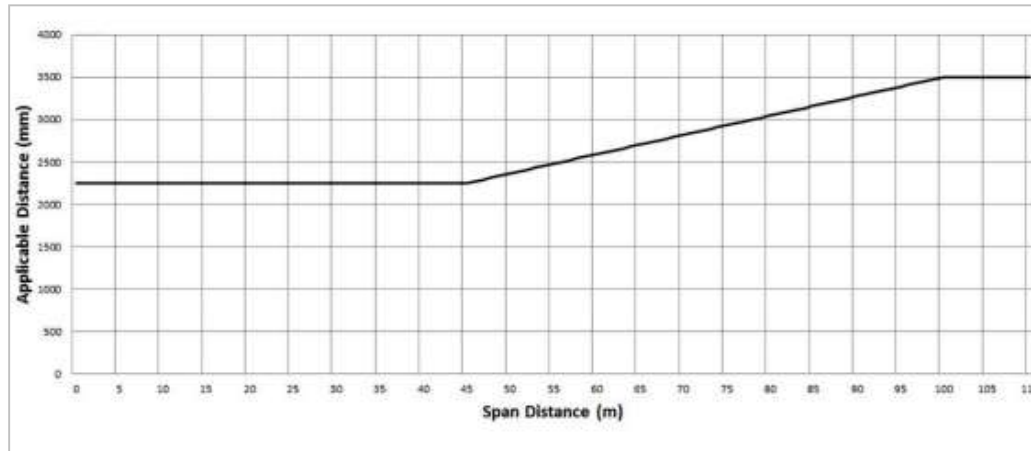
Graph 4: Uninsulated 66,000 Volt Electric Line in Low Bushfire Risk Area
