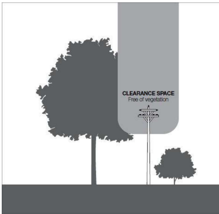
Figure 5 – Uninsulated 66 000 Volt Electric Line in a Low Bushfire Risk Area and Uninsulated Electric Line in a Hazardous Bushfire Risk Area (NOT TO SCALE) Clauses 27, 28 and 29, Graphs 4, 5 and 6
