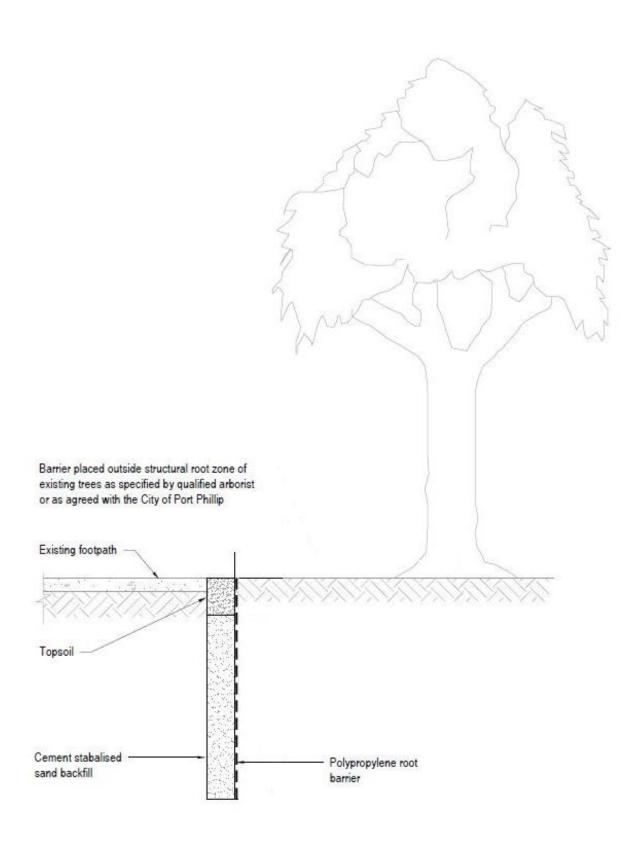
POLYPROPYLENE ROOT BARRIER ELEVATION
