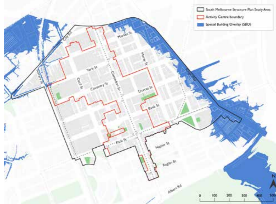
Figure 10 – The Special Building Overlay helps manage development on land in flood prone areas.
