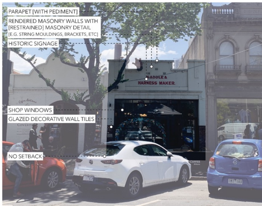
Figure 32. Single-storey commercial building typology, showing typical features.
