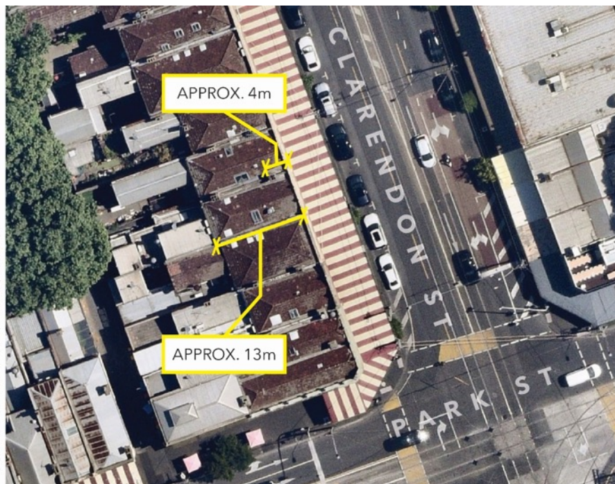
DIAGRAM: TYPICAL RELATIONSHIP BETWEEN CHIMNEYS AND PRIMARY BUILDING VOLUME CORNER CLARENDON & PARK STREETS
