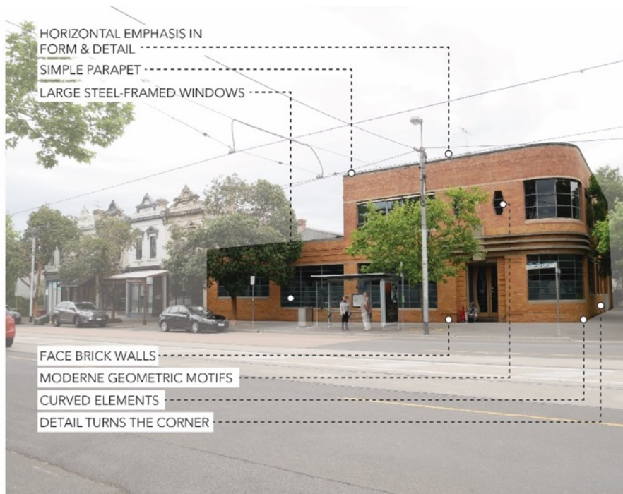
Figure 33. Corner commercial building typology, showing typical features.
