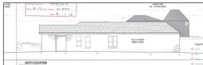
Figure 3. Extract of the endorsed south elevation of 1 Lytton Street, Elwood, illustrating a double-storey boundary wall with a height of approx. 7.7m built on southern boundary (Source: Endorsed Plans, 1 April 2016)
