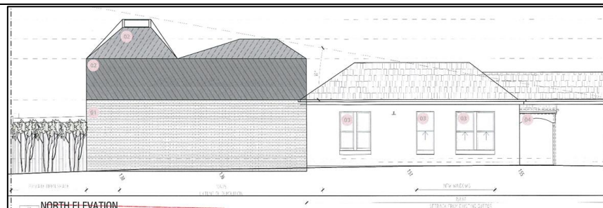
Figure 2. Extract of the endorsed north elevation of 1 Lytton Street, Elwood, illustrating a double-storey boundary wall with a height of approx. 7.7m with a setback of 1.139m (Source: Endorsed Plans, 1 April 2016)
