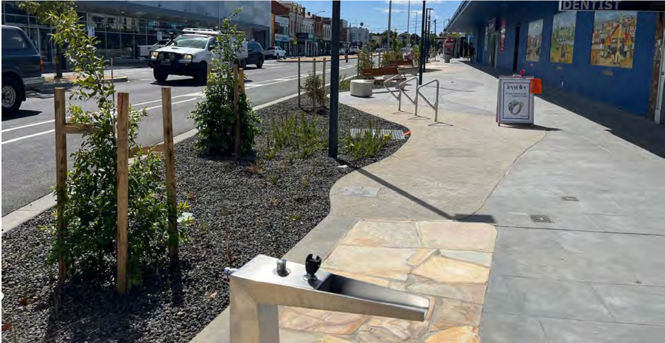
An example of a street that was narrowed, with the additional space being used to widen the footpath and create space for planting in Geelong (Image Credit Revitalising Central Geelong).
