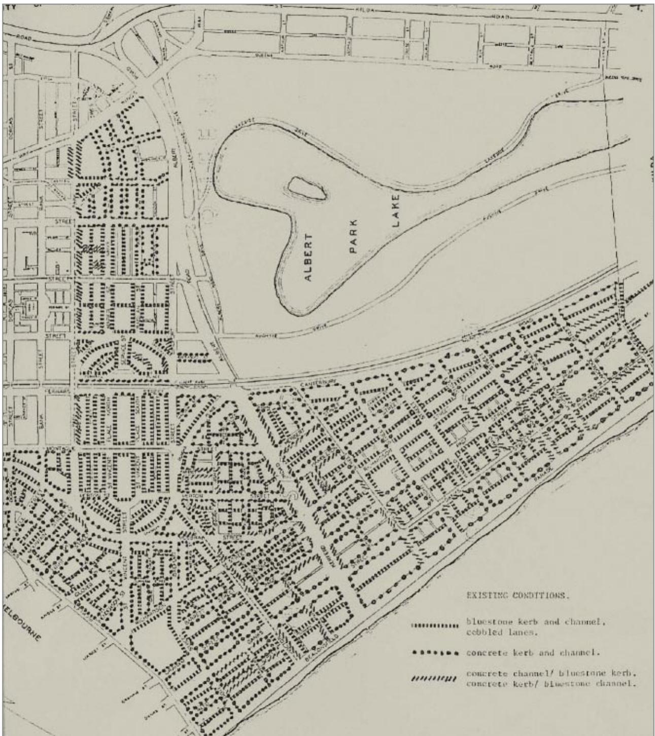
Image 12. 1980 Survey of extant bluestone kerb, channelling and laneways in South Melbourne, Albert Park and Middle Park. Source: Urban Advisory Committee, A Report to the South Melbourne City Council: Bluestone Street Works in South Melbourne, The Urban Advisory Committee, February 1980
