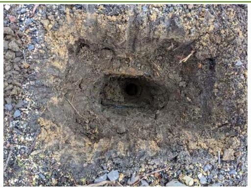
**Photo ID: 5** – Example of 200mm diameter pit within fill material (SB06)
