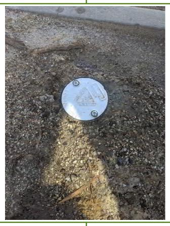
**Photo ID: 10** – Example of installed groundwater monitoring bore (GW03).
