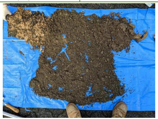
**Photo ID: 6** – Example of soil inspection for fibrous material within fill (SB05)
