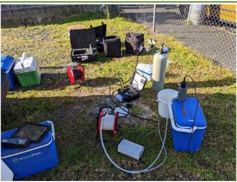
**Photo ID: 9** – Groundwater low flow monitoring set up at GW02.
