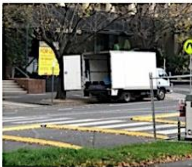
Frequent kerbside parking and drop-offs in close proximity or over mid-block pedestrian crossing impeding pedestrians and safe sight lines of pedestrian movements.
