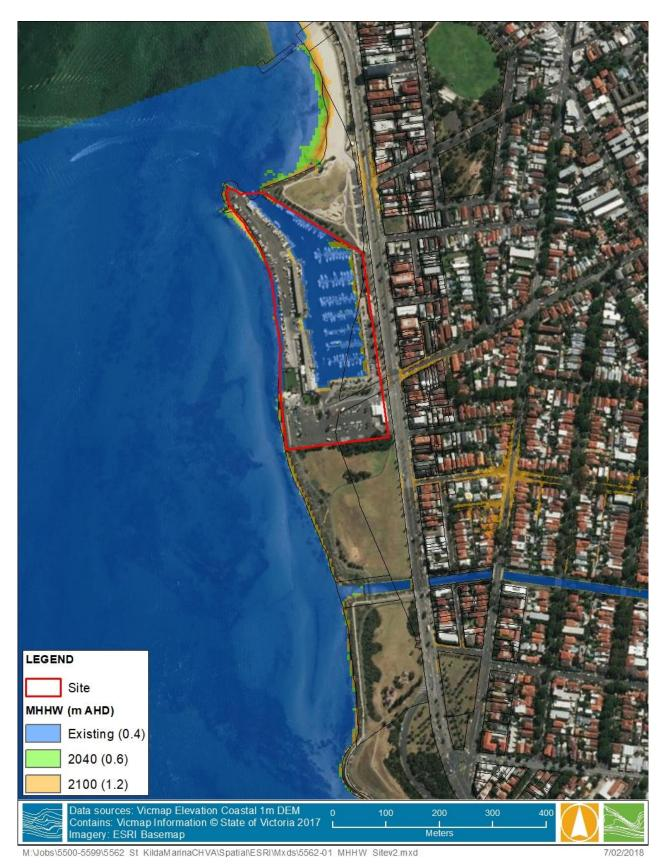
FIGURE F-6 PREDICTED MHHW EXTENT AT ST KILDA MARINA FOR VARIOUS SEA LEVEL RISE SCENARIOS (USING 2009 LIDAR AND 2017 BATHYMETRY SURVEY)
