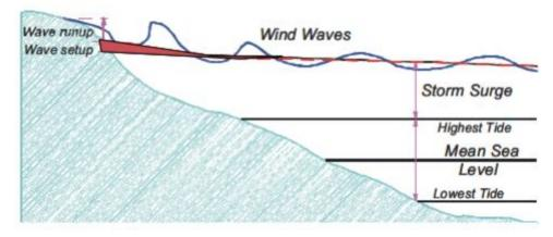
FIGURE F-10 WAVE SET-UP AND RUN-UP (CSIRO 2009)
