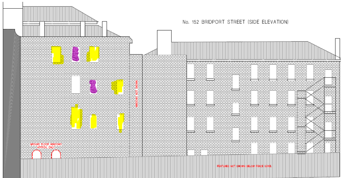
Image 13. Screenshot of east facing habitable Biltmore windows highlighted yellow, non-habitable highlighted purple. Source: Source: Plan of Reestablishment and Detail Survey by JRL Land surveyors. NB: a discrepancy exists as one surveyed window at second floor is not shown on the endorsed plans.
