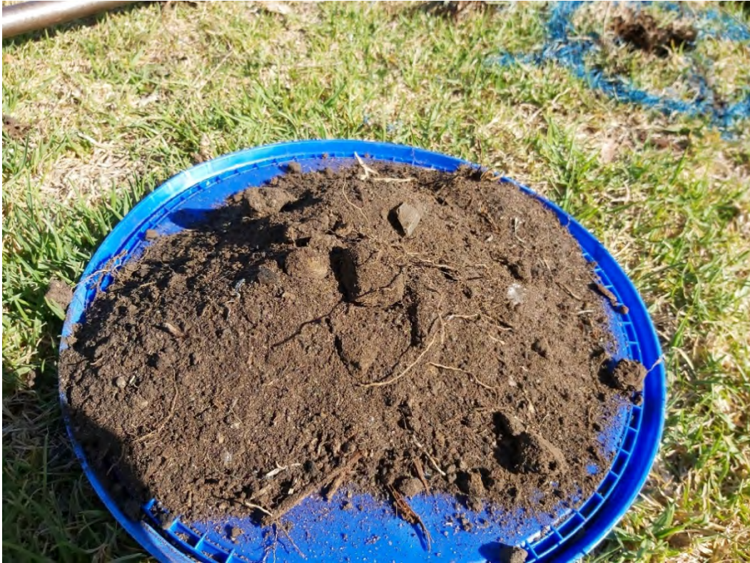
Photo 7. Example of FILL: Silty SAND with gravel and glass fragments at location SB16.
