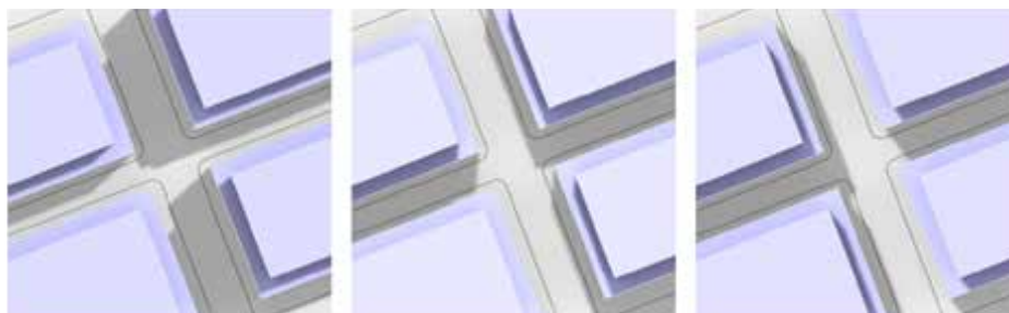
Overshadowing of 20m wide north-south streets at 10.00am, 12.00pm and 2.00pm based on a 4 storey street wall, 5m upper level setback and 6 storey building height for non-residential development.
