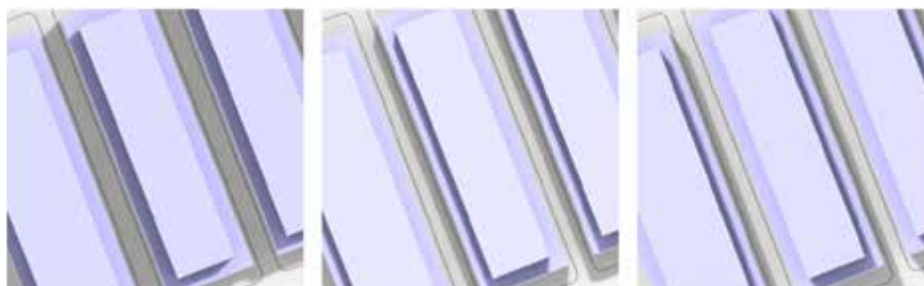
Overshadowing of 9m wide north-south streets at 10.00am, 12.00pm and 2.00pm based on a 3 storey street wall, 5m upper level setback and 5 storey building height for non-residential development.
