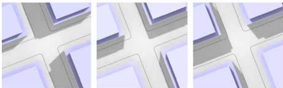
Overshadowing of 30m wide streets at 10.00am, 12.00pm and 2.00pm based on a 5 storey street wall, 5m upper level setback and 7 storey building height for non-residential development.
