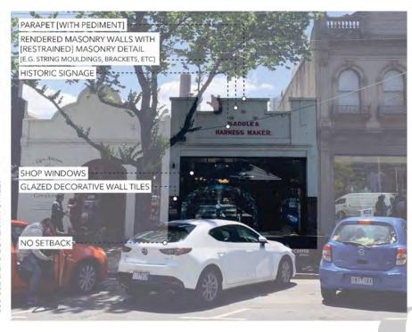
Figure 32. Single-storey commercial building typology, showing typical features.
