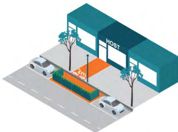
Figure 17: The design of the entrance to the Business Parklet needs to take into account fixed objects in the footpath such as trees and lighting.
