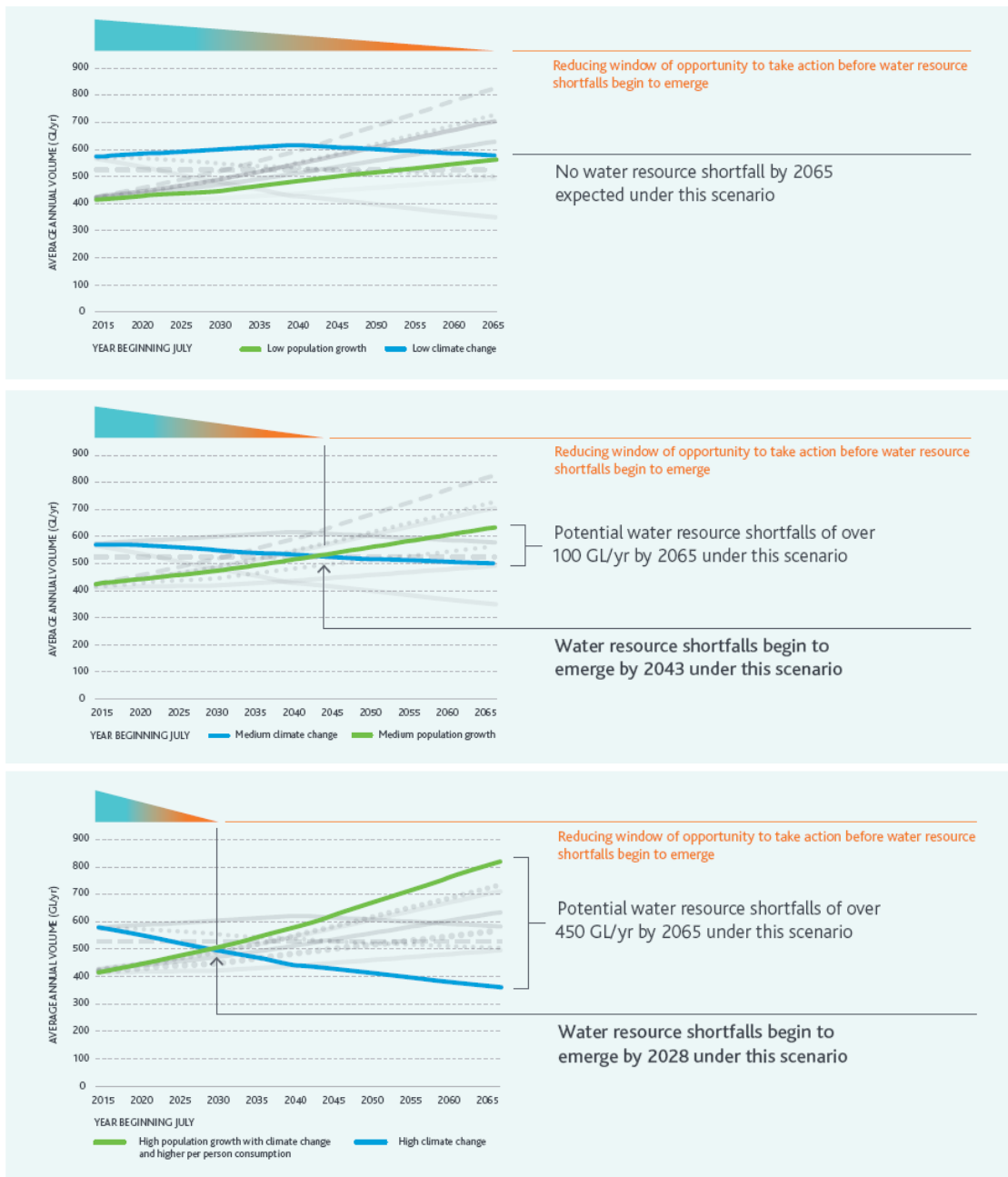
Figure 30: Three key scenarios of supply and demand used during the development of the Melbourne Water System Strategy (2017) this strategy: low change scenario (top), incremental change scenario (middle), and rapid change scenario (bottom) 51
