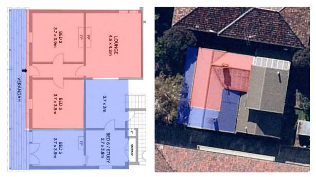
Figures 6 & 7 - Floor plan (left) and recent aerial photograph showing the front part of the house. The original extent of the three-roomed 1872 cottage is shaded red, and the 1890s additions are shaded blue. (Source: McGrath Real Estate and Nearmap)
