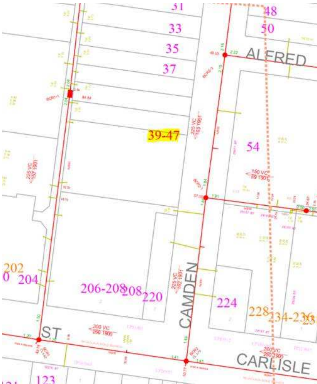
Figure 4-1 Sewer Assets from Dial Before You Dig
