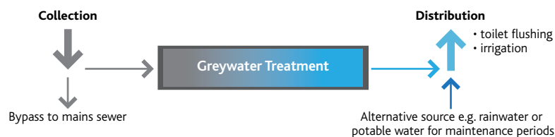
Figure 10. Schematic of greywater reuse system
